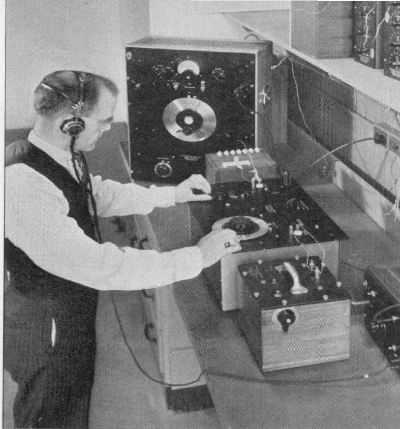
FIGURE 2. Calibrating a TYPE 722 Precision Condenser in the Standardizing Laboratory.
